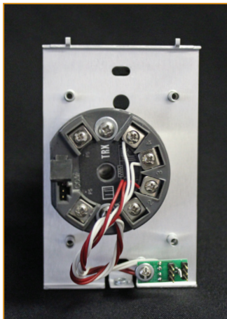
Right: Internal: Transmitter and RTD
